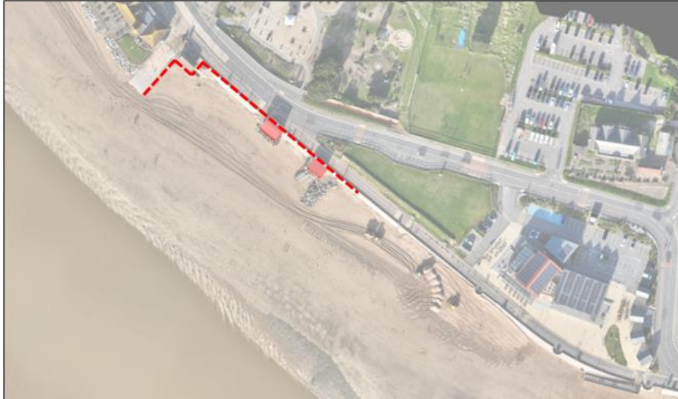
Red Dash – Proposed Pile Alignment Red Area – Possible building removal to elsewhere
